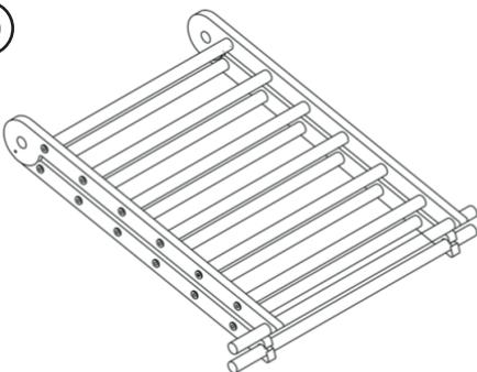
Insert one of the longer, bottom rungs (A) through the hole at the bottom of one of the legs and push through to the corresponding hole on the opposite leg.
