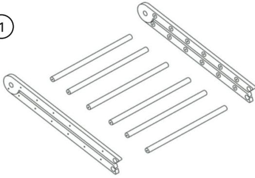
Lay out the leg assemblies and six of the shorter rungs (C) roughly as above. Place the legs with the larger holes facing inwards.
