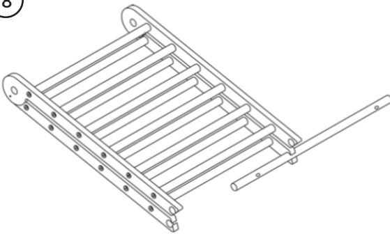
Insert one of the longer, bottom rungs (A) through the hole at the bottom of one of the legs and push through to the corresponding hole on the opposite leg.
