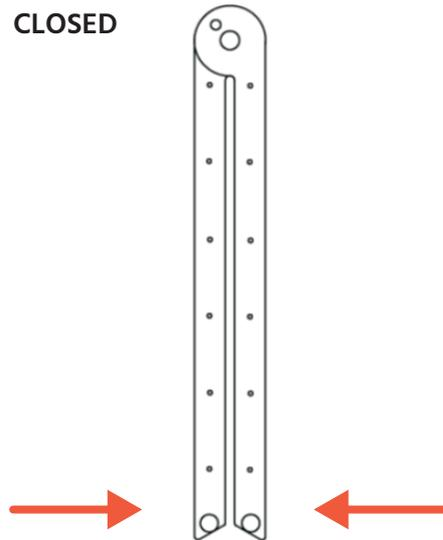
Your Tri Climb includes two thumb screws that are designed to lock the product in an open or closed position.
