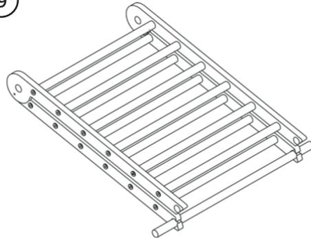
Line the countersunk holes on the bottom rung (A) up with the centre of the frame legs (C). Insert the two screws (E) and carefully, with controlled force, screw into the frame and tighten using a screwdriver. Be careful to ensure screws are centre to frame.
