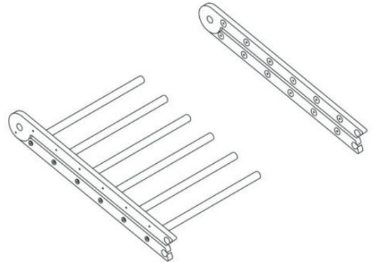
Insert rungs into recessed holes on one side. Insert flat head screws (D) and tighten using the hex key provided.
