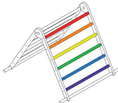
Open the Triclimb frame and stand it up. If the frame is not quite sitting flat on the floor, repeat the procedure in step 6, placing downward pressure on the frame until it sits completely flat.
