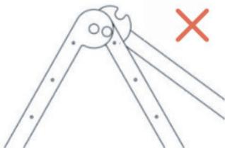
**WARNING:** Must not be placed on the very top rung of the Triclimb. It must be connected between two rungs with one rung above and one rung below in order to lock.
