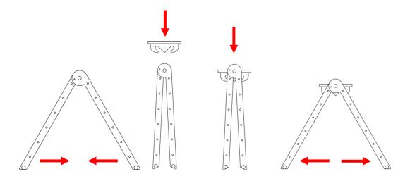
**STEP 1**No tools are required. Simply close the Triclimb to almost closed.
